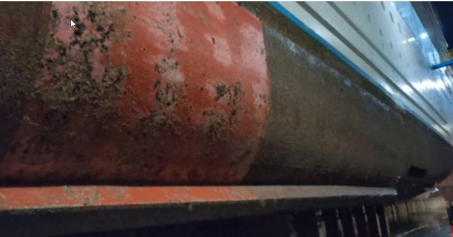
Figure 3.7 Biofouling attached to hull and antifouling to protect it (source Marine Insight)
